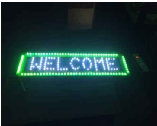
Welcome board by soldering LED bulbs in series by 8 th Std students
